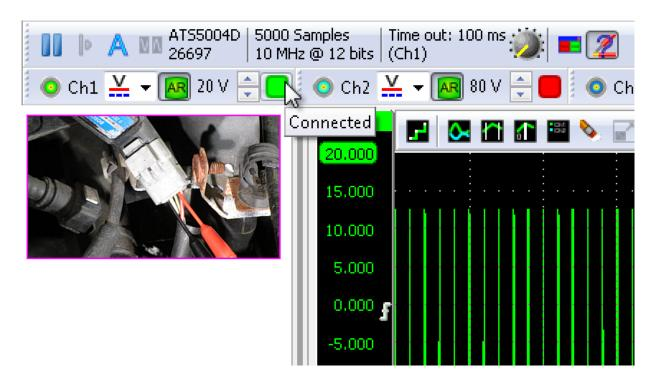
As can be seen in a video on our website, capacitive coupling between test probe and test subject can result in measuring a distorted version of the actual signal, wrongly suggesting a connection. SureConnect however immediately shows you whether a good connection is present.
