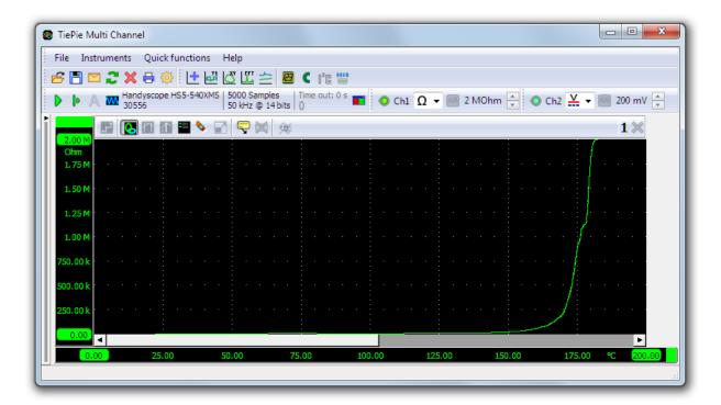
The Ohm scope uses the same inputs as the oscilloscope. Changing the measure leads is not required. The advanced protection against over voltage ensures that the Ohm scope withstands high voltages.
