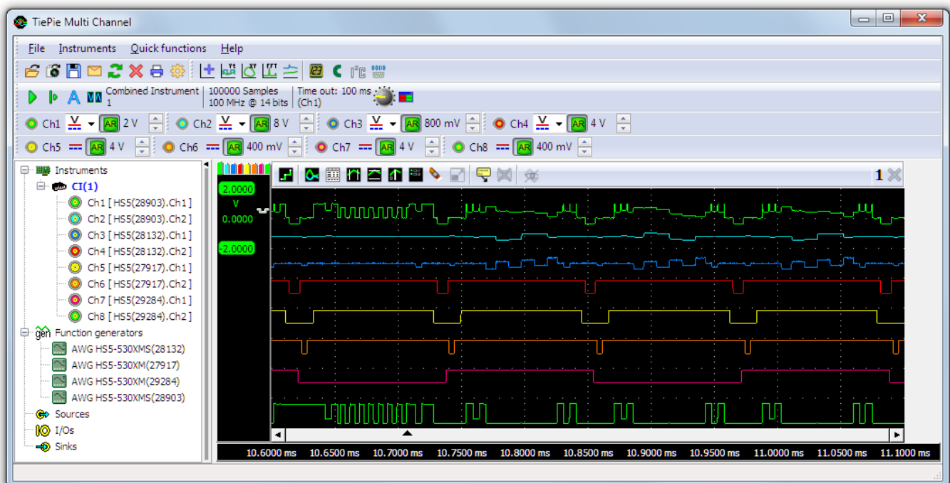
Figure 2: Four Handyscope HS5s combined to an 8 channel 12 bit 500 MS/s oscilloscope
