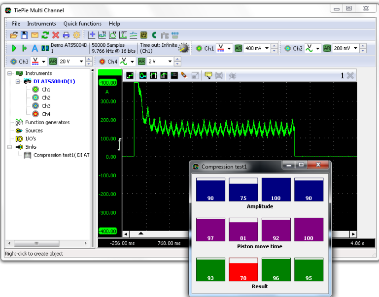
Figure 9.5: Compression test on engine with leaking cylinder
