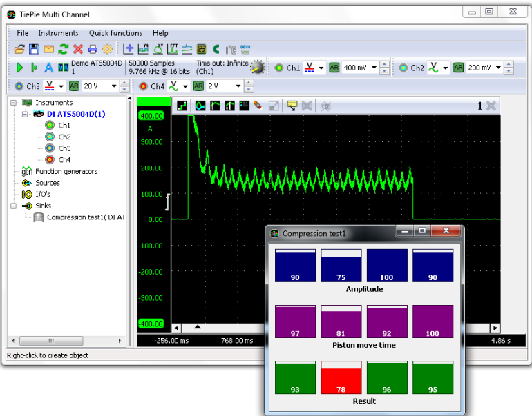
Figure 9.5: Compression test on engine with leaking cylinder
