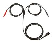
The Measure lead TP-C1812B is a low noise differential measure lead designed to be used with the Handyscope HS4 DIFF and the ATS5004D. This 3 meter long measure lead splits in two individual ends of each 1.2 meter long. The BNC connector at one end plugs directly on the instrument. The two other ends each feature a single 4 mm banana jack, on which application specific test points, clamps or probes can be plugged.
