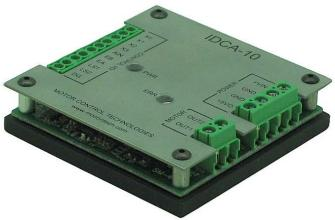
The IDCA-10 is an integrated servo control system designed specifically for DC brushed motors. MCT brings a unique solution to motor control with this innovative product. The IDCA-10 possesses a dedicated PID control loop, localizing control functions on the motor hardware. The IDCA-10 is designed with flexibility in mind and is easily configured for a number of different operating modes. Operating modes include:
