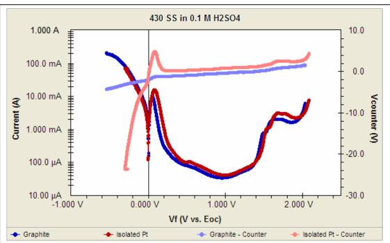
Figure 2. The current voltage curves for 430 Stainless Steel in 0.1M H<sub>2</sub>SO<sub>4</sub>. The darker curves are the current voltage data. The lighter curves are the control amplifier output recorded at the same time. Blue: graphite counter electrode. Red: isolated Pt counter electrode.
