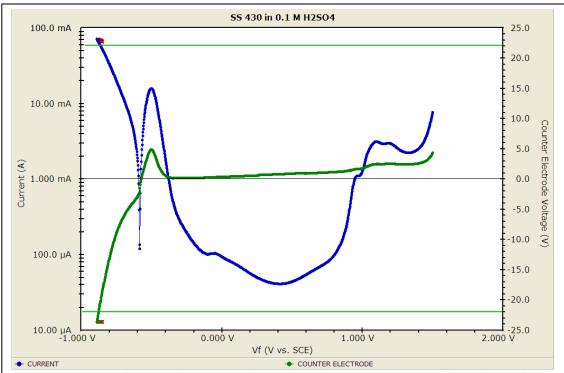
Figure 4. Current (blue) and Counter Electrode Voltage (green) vs. Working Electrode Voltage. The horizontal green lines mark the published compliance voltage limits of the potentiostat: ±22 V. Red marks points with a "Control Amplifier Overload."
