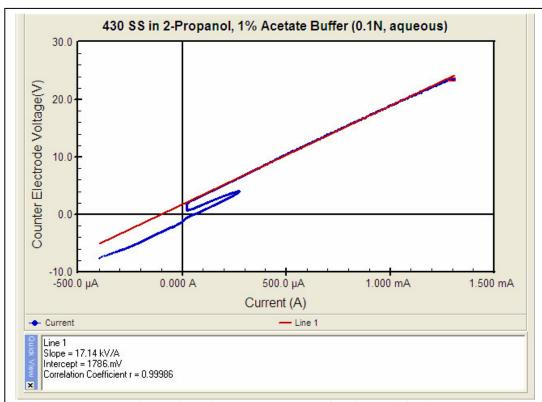
Figure 6. Counter Electrode Voltage vs. Current. The slope of the least squares fit gives the bulk resistance of the solution, 17.14 kohms.
