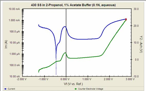
Figure 5. 430 Stainless Steel in 2-Propanol to which 1% aqueous 0.1N Acetate Buffer had been added. This mixture approximates an alternative fuel mixture. Experimental details: Gamry EuroCell™, Graphite rod counter electrode (not isolated), SCE Reference Electrode, Ref. Electrode Bridge Tube filled with isopropanol electrolyte.
