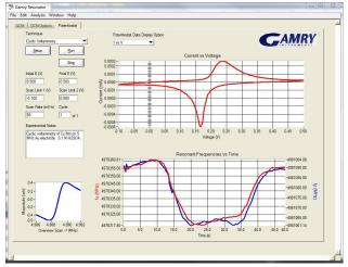
*Frequency data are also displayed on the potentiostat tab during acquisition.* Here are both the OCM and potentiostat responses during the cycling of a Cu film on an Au electrode.
