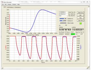
**Data acquisition is controlled with one program.** QCM control is on one tab while potentiostat control is on another tab.
