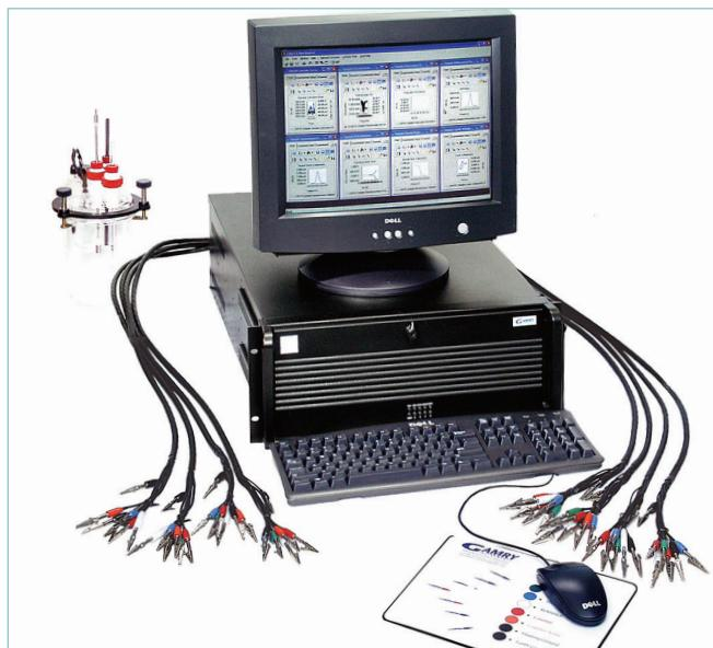
cells. The ECM8 converts a single Potentiostat into a powerful instrument suitable for automating repetitive electrochemical experiments in a sequential fashion.
