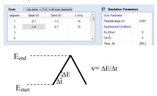
**CV setup and anatomy of the CV signal** Three parameters define the signal.  $E_{start}$ ,  $E_{end}$ , and sweep rate are available on the setup screen as shown.
