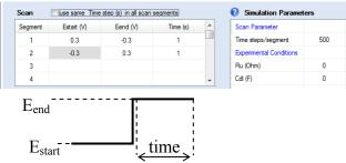
**CA setup and anatomy of the CA signal** Three parameters define the signal.  $E_{start}$ ,  $E_{end}$  and time are available on the setup screen as shown.
