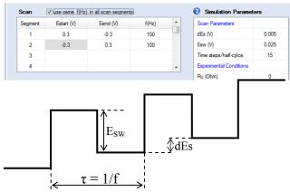
**SWV scan setup and anatomy of the SWV signal** Three parameters define the signal. f,dE<sub>s</sub> and E<sub>sw</sub> are available on the setup screen.
