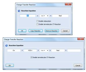
**Reaction Setup Dialog Box** The reactions can be fully reversible or irreversible with multiple electrons. If "Enable Adsorption" is selected, the "Surface Reactions" tab will be enabled. If the "Enable termolecular CT-Reaction" toggle is selected, the dialog box changes to the second box above.
