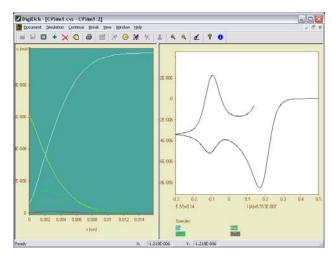
The concentration distance curve An evolving concentration distance curve will be shown concurrent with the CV.
