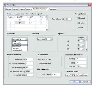
Setup Screen for the Simulation Parameters Electrode geometry, dimensionality, pre-equilibria, and a range of computational parameters
