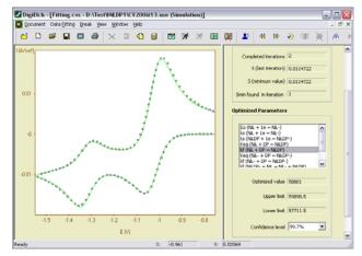
CV fitting A group of data files, imported into DigiElch can be fit to a mechanism.
