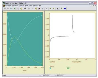
**CA simulation and concentration profiles** ChronoAmperometry and concentration profiles can also be simulated with any of the systems described in the CV section
