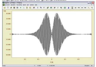
FT Simulation result The result of the simulation provides the DC current as well as the fundamental and higher harmonic AC response.
