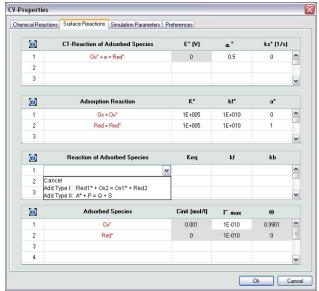
Surface Reactions Setup Tab DigiElch 6 can be used to simulate adsorption-desorption and surface reactions with unprecedented detail
