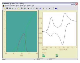
The coverage potential curve The coverage of the surface adsorbed species can be displayed as a function of potential as percent coverage of the  $\Gamma_{max}$  entered during setup.
