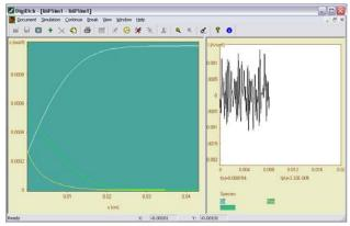
**IMP simulation** The IMP signal is applied in time domain where the concentration profiles can be plotted in an evolving fashion.
