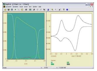
CV and concentration potential profiles The simulations can include adsorbed species as well as species diffusing from solution.
