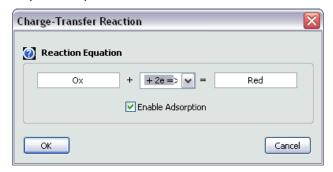
**Reaction Setup Dialog Box** The reactions can be fully reversible or irreversible with multiple electrons. If "Enable Adsorption" is selected, the "Surface Reactions" tab will be enabled.
