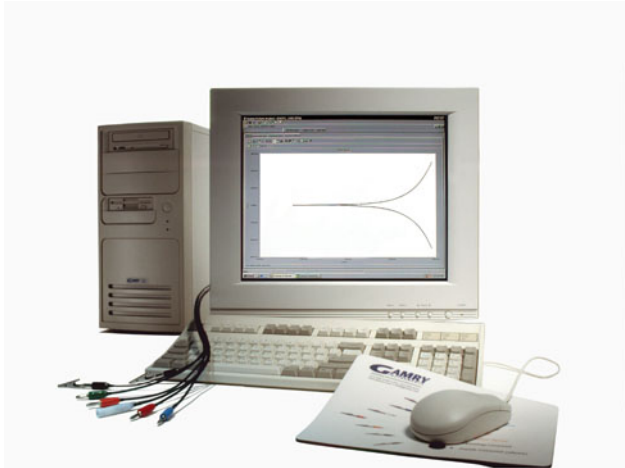
The DC105 Corrosion Techniques Software in a Windows-compatible computer controls a Gamry Potentiostat to perform the electrochemical corrosion measurement.
