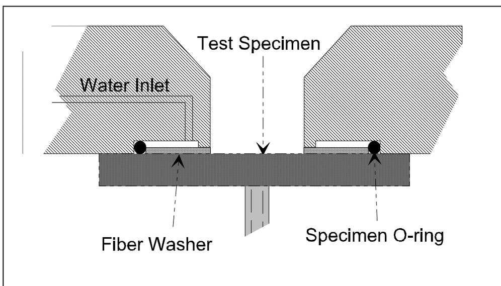
As in conventional cells, the active area of the test specimen is in contact with an electrolyte. Unlike other cells, the active area of the test specimen is not bounded by a plastic barrier or O-ring.
