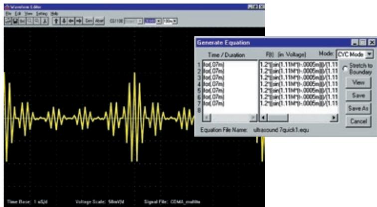
CGWin lets the user create arbitrary waveforms either by Equation Entry or by loading signal files. These waveforms can then be output through a CompuGen ISA signal generation card.
