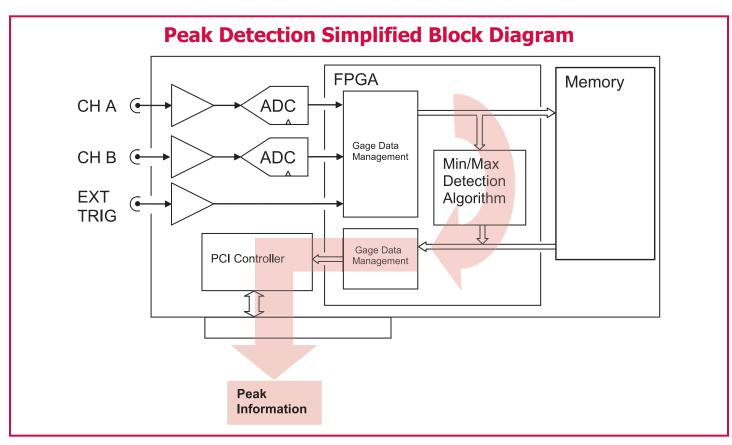
The Peak Information Set contains the minimum and maximum peak values within a waveform data set. These peak values are the absolute peak positions of the waveform when the peak occurs and the on-board time-stamping counter indicates the time of the occurrence. The list of parameters that comprise the Peak Information Set is shown in the table below:
