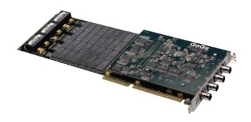
Arbitrary waveform generator and function generator card capable of providing aperiodic analog waveforms.
