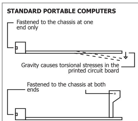
This redundancy in retaining the cards provides tremendous improvement in mechanical ruggedness of the entire instrument, particularly for mobile applications and during transport.
