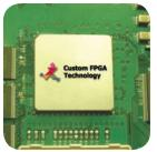
**Advanced eXpert on-board signal analysis features** such as GaGe's Signal Averaging, FIR Filtering, Fast Fourier Transform (FFT), and Peak (Min/Max) Detection are optionally available on GaGe's new-generation high-performance PCI digitizer cards as Field Programmable Gate Array (FPGA) images. These features provide a fast and efficient means for users to process data on-board GaGe's digitizers and transfer only the data that is of interest to the PC for further analysis.
