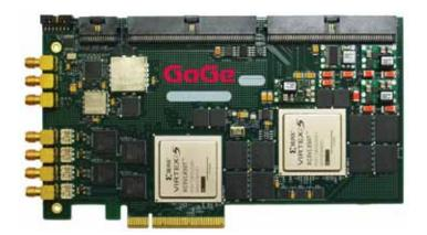
Arbitrary waveform generator and function generator PCIe card capable of providing high-speed aperiodic analog waveforms.
