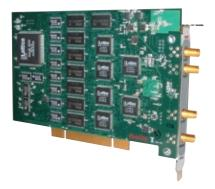
Arbitrary waveform generator and function generator card capable of providing aperiodic analog waveforms.
