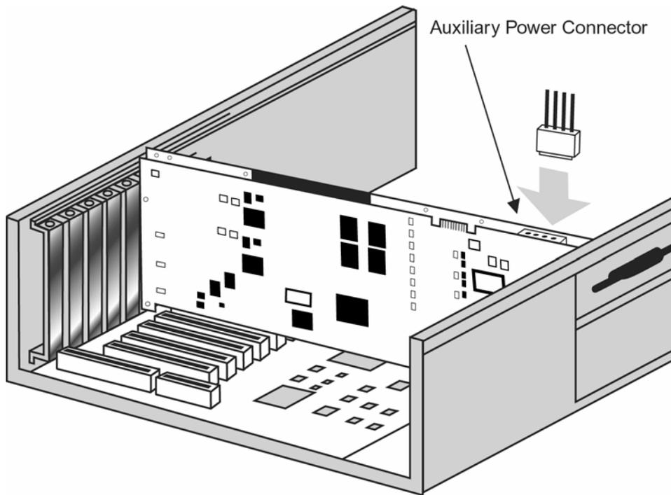
*Figure 11: Connecting auxiliary power: single card*
