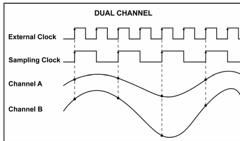
*Figure 30: CS12100, CS1250, CS1610, CS1602\* Dual channel External Clock*
