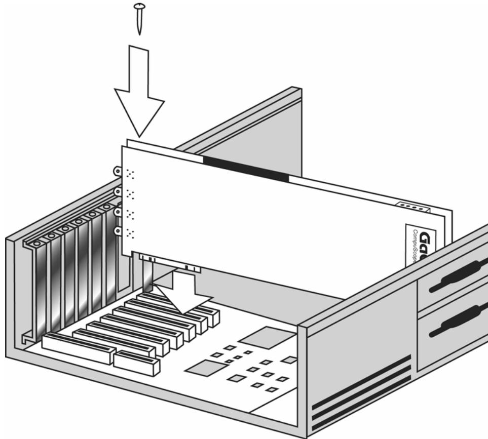
*Figure 10: Inserting a single card*
