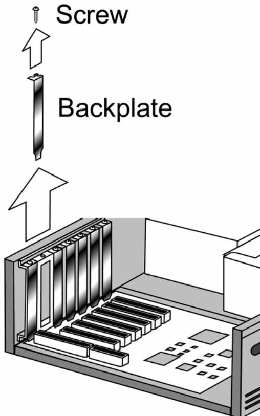
*Figure 15: Removing the backplate*
