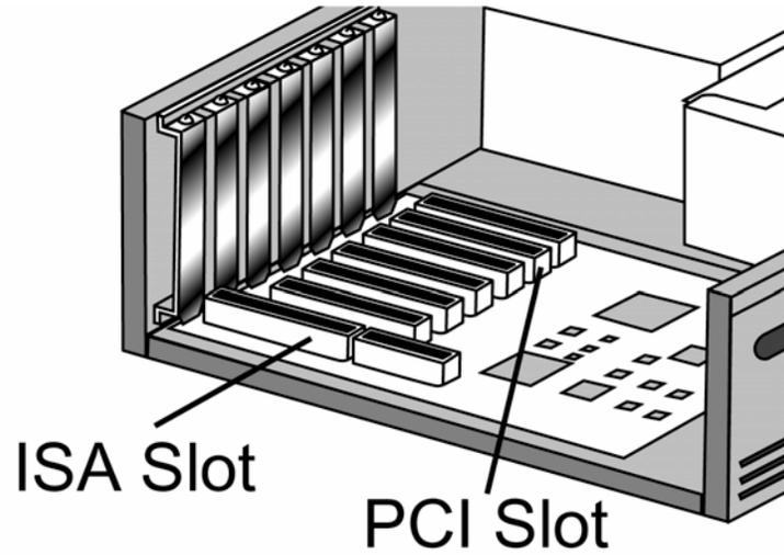
*Figure 8: Selecting a PCI slot*
