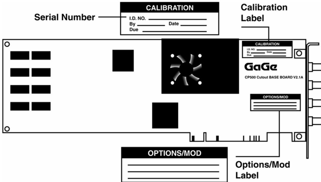
*Figure 3: Calibration label and OPTION/MOD label*
