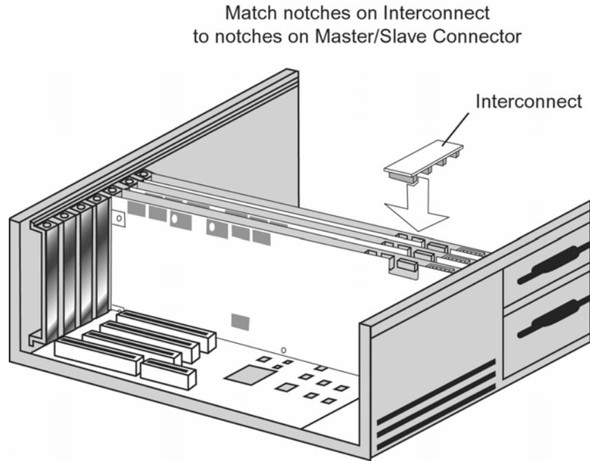
**Figure 18: Installing MSTM for CompuScope 12100, 1250, 1220, 1602, 1610 or 3200**
