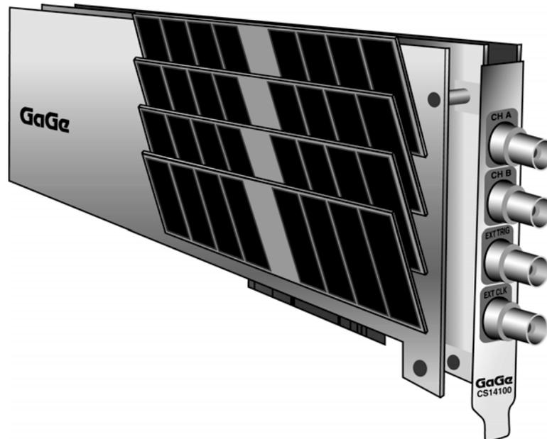
*Figure 6: CompuScope card with Deep Memory Board*
