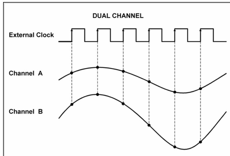
*Figure 29: CS82G, CS1220, CS14200, CS14105, CS14100 & CS1450 Dual channel External Clock*
