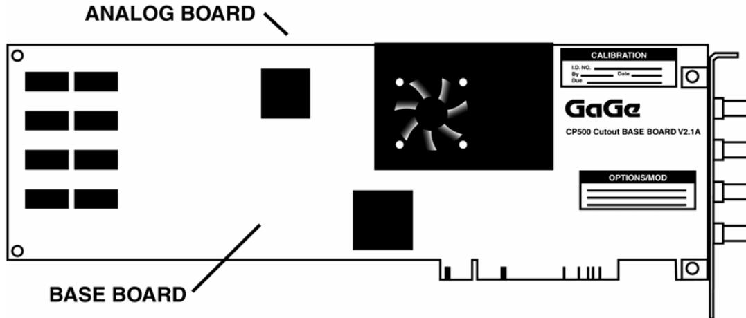
*Figure 1: CS12100 and CS1250 base board and analog board*
