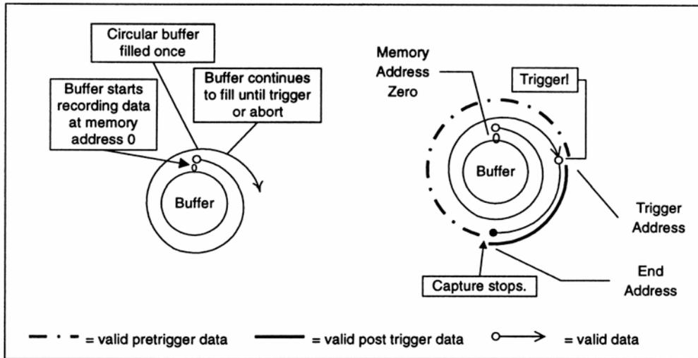
*Figure 32: Pre-Trigger: all data points in buffer valid*
