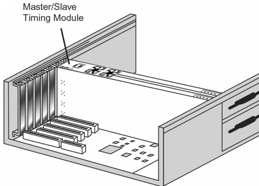
**Figure 19: Installing MSTM for CompuScope 82G, 8500, 14100 or 1450**
