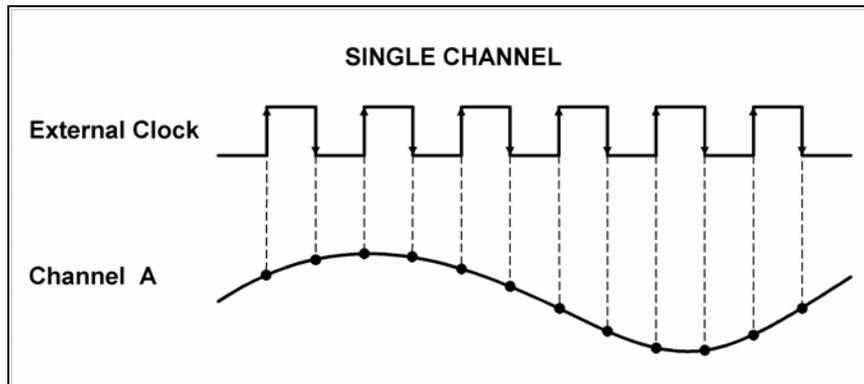
*Figure 28: Single channel External Clock on the CompuScope 82G*
