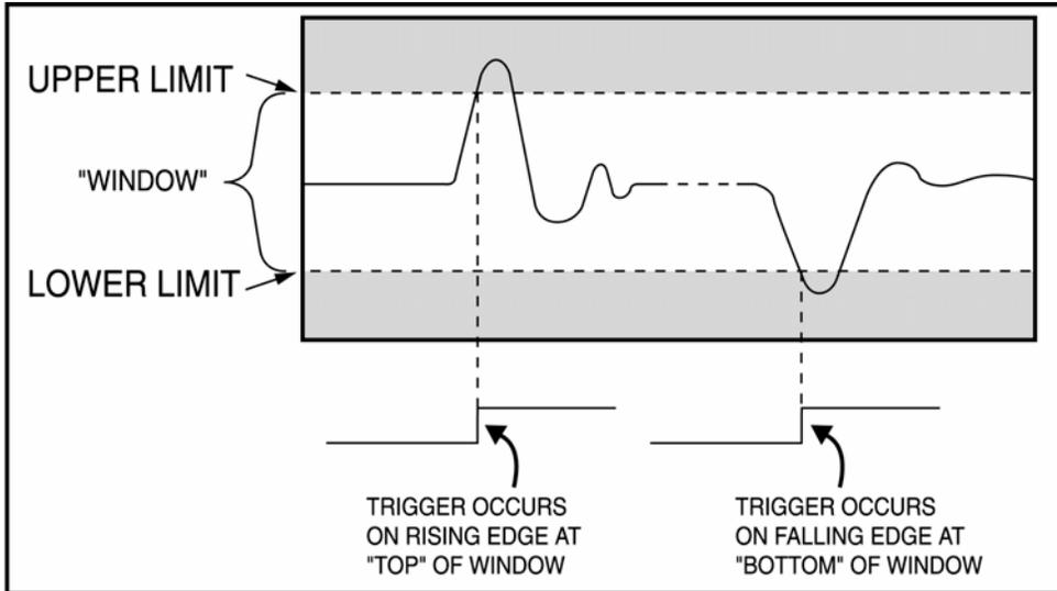
Figure 24: Windowed triggering
