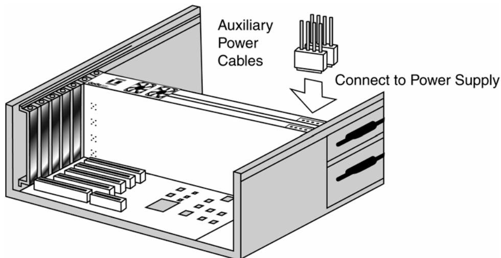
*Figure 21: Connecting auxiliary power cable on CS8500, CS14100 or CS1450 multi-card systems*
