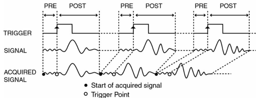
**Figure 26: Multiple Record mode with Pre-Trigger data**
