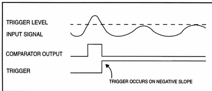
*Figure 23: Generation of a trigger signal – negative slope*
