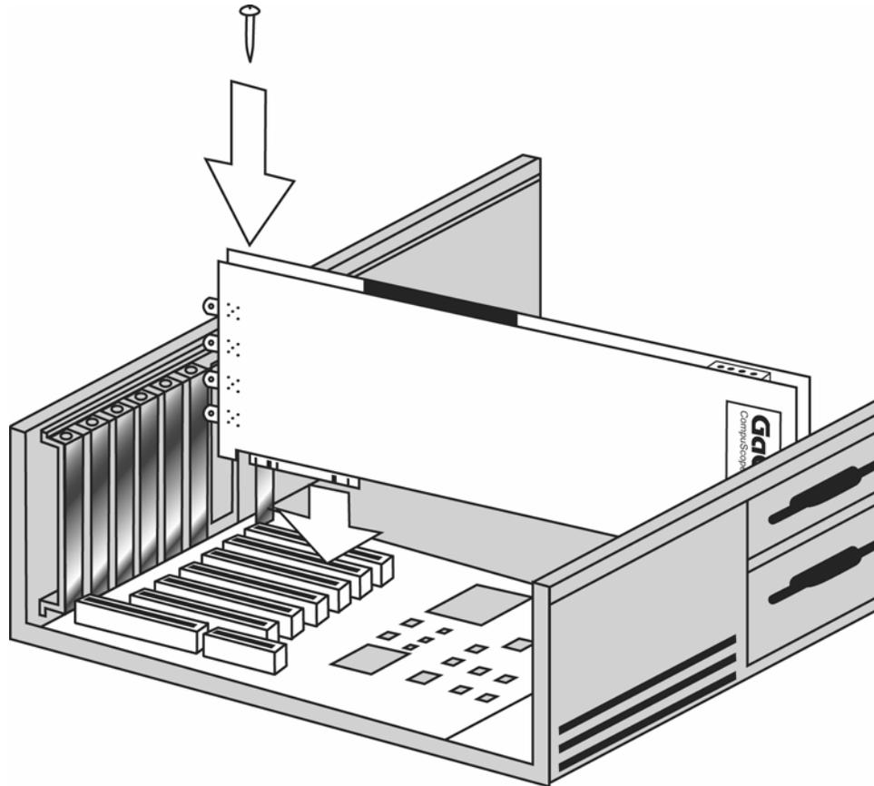
*Figure 16: Installing the Master card or the first multiple independent card*
