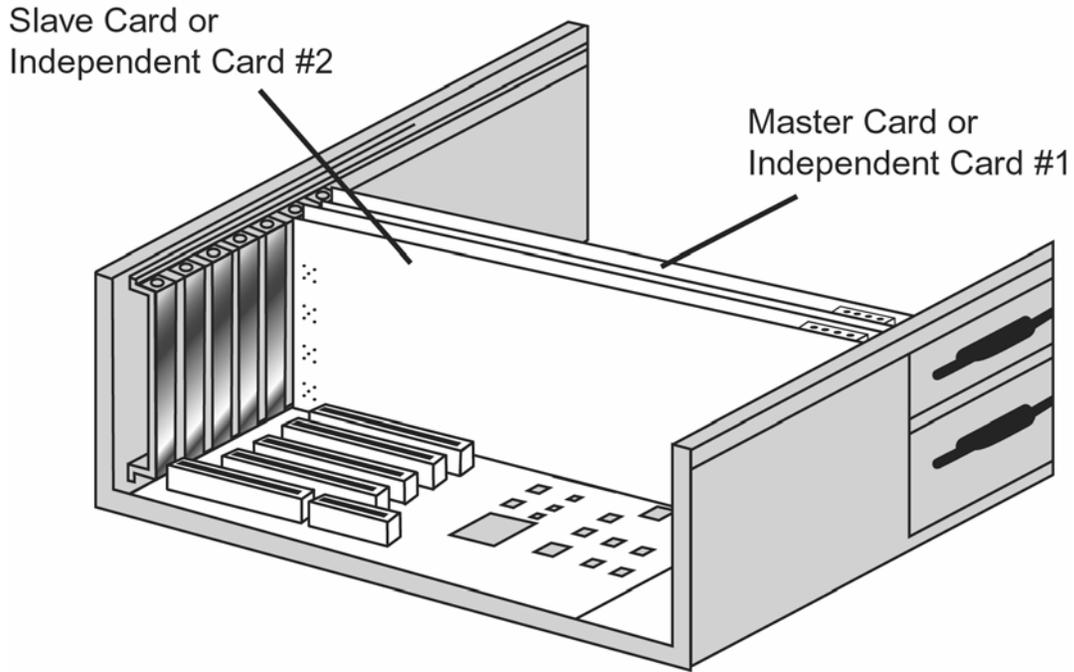
*Figure 17: Inserting multiple CompuScope cards*
