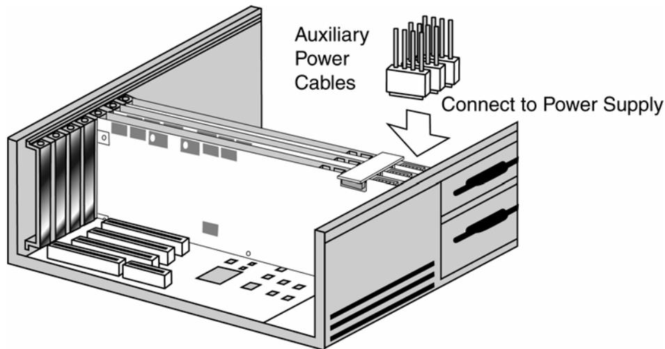
*Figure 20: Connecting auxiliary power cable on CS12100, CS1250, CS1220, CS1602 or CS1610 multi-card systems*
