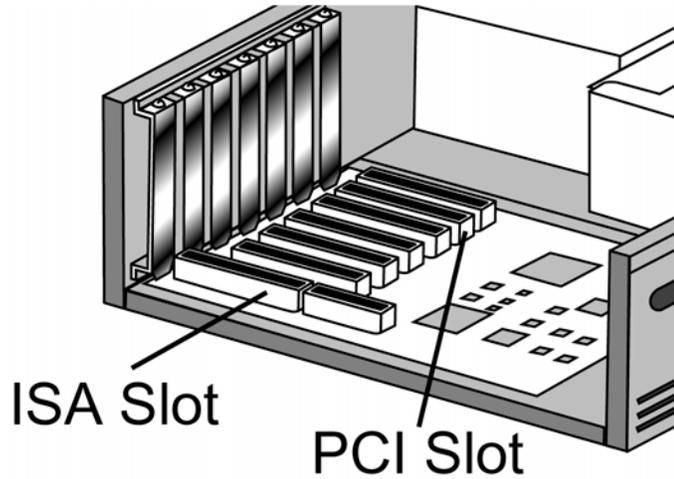
*Figure 14: Selecting PCI slots*
