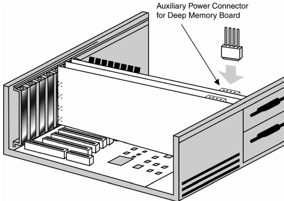
*Figure 12: Connecting auxiliary power connector for 64M and higher memory models*
