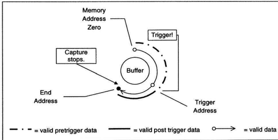
*Figure 33: Pre-Trigger: not all data points in buffer valid*
