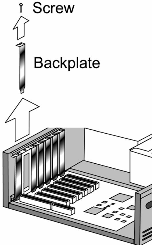
*Figure 9: Removing the backplate*
