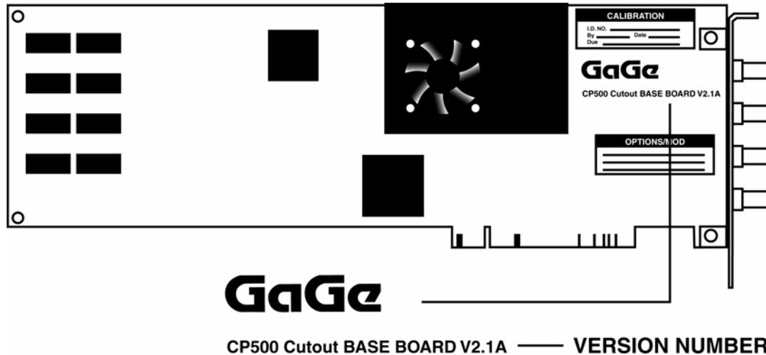
*Figure 2: Base board hardware version number*
