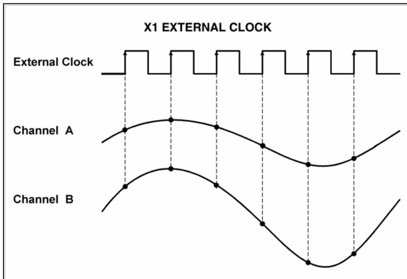
Figure 31: X1 External Clock upgrade in dual channel mode
