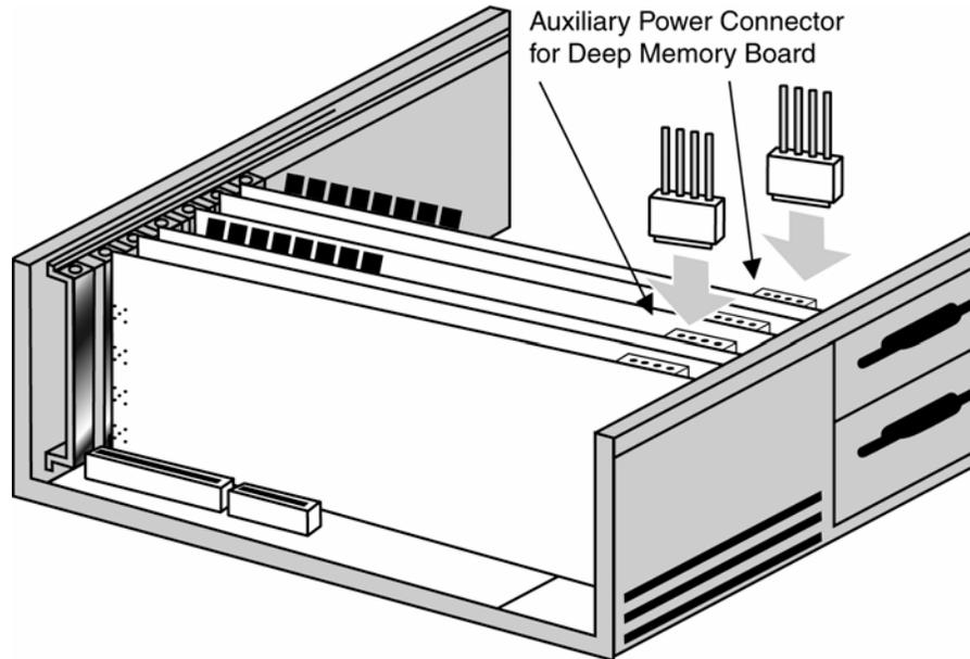
*Figure 22: Connecting auxiliary power connector for multi-card systems with 64M and higher memory models*
