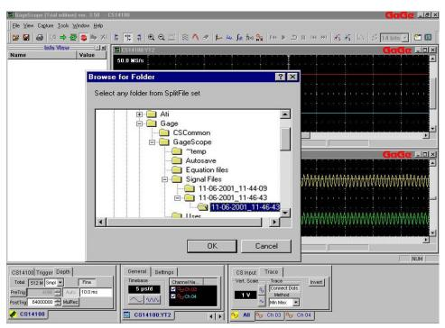
16 GageScope<sup>®</sup> confirms the Split File structure and asks for confirmation:
