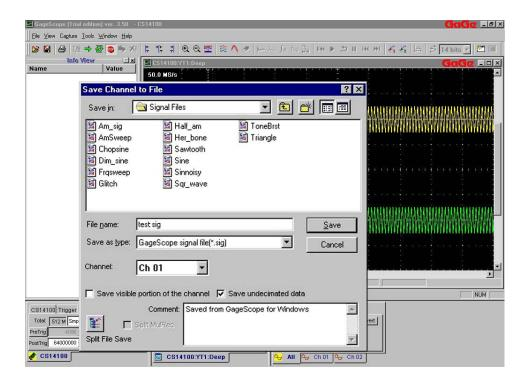
As already indicated on the dialog, click the "Save undecimated data" checkbox, choose which channel to save (Ch. 01 in this case), enter a name for the file ('test' in the case of the example), select a location for the file, and then click on Save.
