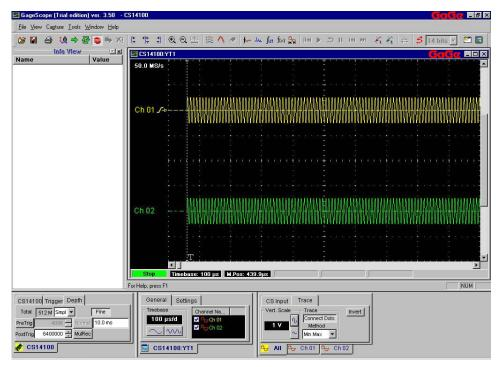
While computers may have a varying amount of RAM, in GageScope<sup>®</sup> the **DM Buffer** size must be between 1 and 64 megabytes so as to ensure smooth operation on the vast majority of PCs. Because the DM Buffer implicitly controls the decimation factor used by GageScope<sup>®</sup>, care must be exercised in specifying a value for the **DM Buffer** size.
