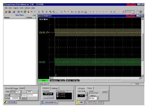
The decimated view is useful to identify the location of peaks in the signal (particularly when using the **MinMax** method) or large-scale patterns in the data. From this summary view, GageScope<sup>®</sup> provides a powerful way of "zooming-in" on the areas of the captured data that may be of particular interest.
