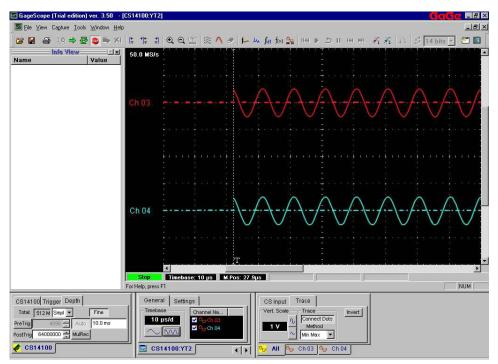
The **DMZ** is used to query the CompuScope board for a segment of captured data without requiring decimation. For this reason, the segment to be fetched and displayed is limited in size to 16 MS and appears disconnected from the complete signal and particularly from the real trigger location. Thus the importance of assigning a position to the **Virtual Trigger**.
