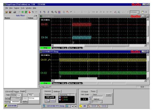
Note the presence of the cursor in the decimated view, with the name 'YT2' displayed in the gray 'range' bar at the bottom. This allows you to quickly identify which position and range of the decimated signal has been zoomed into.
