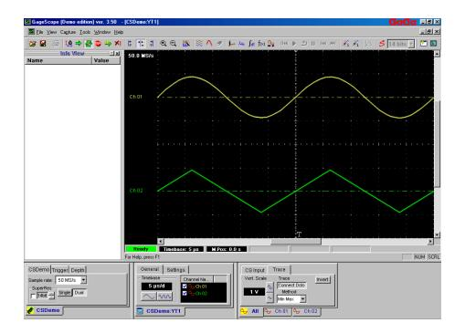
Should you choose not to use these files, you can, however, also load and save disk-based GageScope<sup>®</sup> files (extension .SIG). To load a file, click on File  $\rightarrow$  Load Channel. Sample .SIG files are located in the Signal Files folder inside the C:\Gage\GageScope folder.
