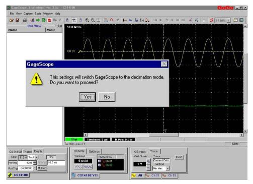
The Decimation Mode is enabled as soon as the size of acquisition per channel is more than  $\frac{1}{4}$ <sup>th</sup> of the size of the **DM Buffer**. For instance, let us assume that you have allocated 8 MB for the **DM Buffer**. In this case, the Decimation Mode will be automatically activated whenever you specify more than 2 MB of total acquisition length in GageScope<sup>®</sup>. The total acquisition length is the sum of the pre- and post-trigger data sizes.
