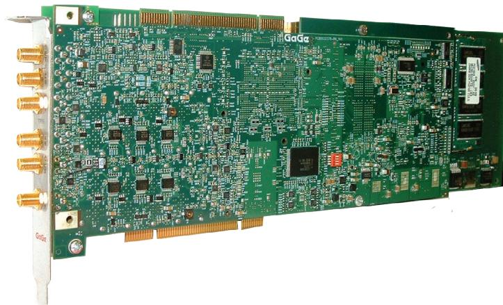
The Cobra CompuScope family is a new generation of GaGe high-speed 8-bit digitizers that provides the most powerful combination of speed, memory, and bandwidth as well as a wide portfolio of advanced acquisition features.
