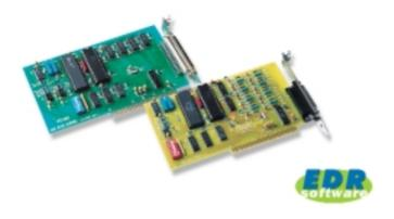
The PC-60 and PC-61 are low-cost, low-speed mA and mV converter boards. They are particularly well designed for use in electrically noisy industrial control systems where fast data acquisition rates are not required. Each board comes supplied with demo software for testing and demonstrating features operation.
