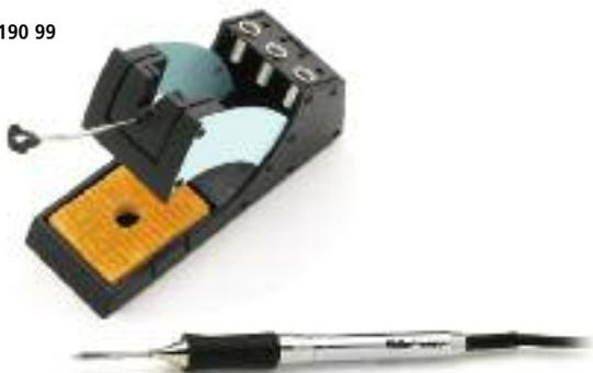
The RT soldering tips have an extremely short heat-up time. All component parts of the system, such as the sensor and heating element, are designed for optimum heat transfer. This ensures absolute efficiency in the utilization of the power provided by the supply unit. The recovery time is minimized. Changing soldering tips is quick, easy, and, most importantly, requires no tools. WMRP set, consisting of WMRP soldering pencil, RT 3 soldering tip and WDH 50 Safety rest.
