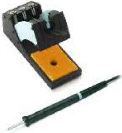
The 65 W micro pencil is up to the task with superior performance for both heat-up and thermal efficiency. Suitable to handle all micro components and fine pitch tasks. The WMP provides an extremely short tip-to-grip distance. The heater is integrated into the handle. When the tip wear out the heating element goes on. WMP set consisting of WMP micro soldering pencil and WDH 20 Safety rest.
