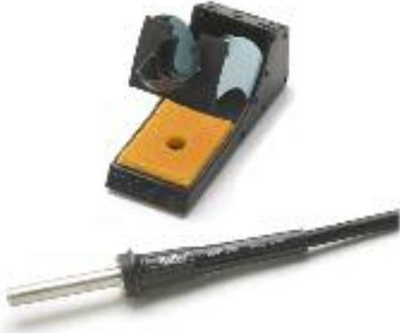
The HAP 200, 200 W/24 V, provides a directional hot airflow that is adjustable and static-free. Electronically temperature controlled from 50°C to 550°C. Different nozzles available as accessories. Finger switch controls speed adjustable pump. Hot air pencil set, consisting of HAP 200 with finger switch, WDH 30 Safety rest for pencil, nozzle 1,2 mm and 3,0 mm, key and nutdriver for nozzle changing.
