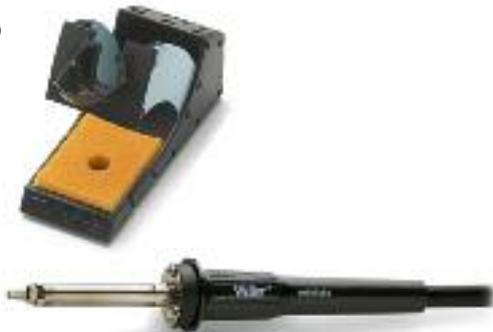
The HAP 1, 100 W/24 V, provides a directional hot airflow that is adjustable and static-free. Electronically temperature controlled from 50°C to 550°C. Different nozzles available as accessories. Finger switch controls speed adjustable pump. Hot air pencil set, consisting of HAP 1 with finger switch, WDH 30 Safety rest for pencil, nozzle 1,2 and 3,0 mm, key and nutdriver for nozzle changing.
