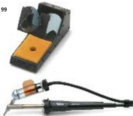
An 80 W/24 V desoldering iron for electronics rework. Electronically temperature controlled. Micro-finger switch controls quick-start, fast action vacuum pump. Different interchangeable tiptets, plus several CSF devices are available as accessories. DSX 80 set, consisting of DSX 80 Desoldering iron, WDH 30 Safety rest, cleaning tool, glass collector, two desoldering nozzles, gasket, anti-bloc paste, filter.
