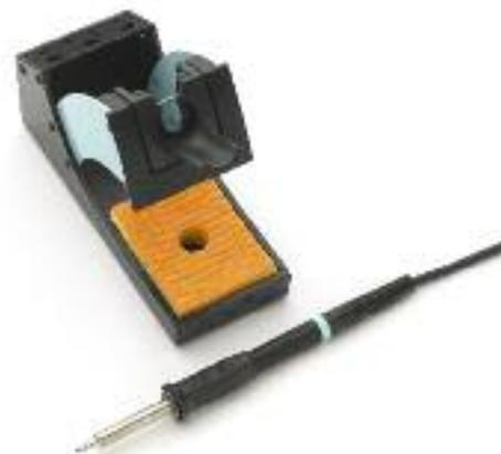
The 80 W micro soldering pencil WP 80 persuades with its short tip-to-grip design, being of big advantage for work under microscopes. The distance from grip to the tip is 40 mm only. WP 80 set, consisting of WP 80 soldering pencil and WDH 10 Safety rest.
