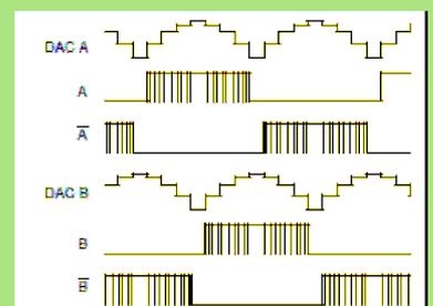
Note that feedback will change the PWM signal to maintain a sinusoidal current, and this may add additional pulses.
