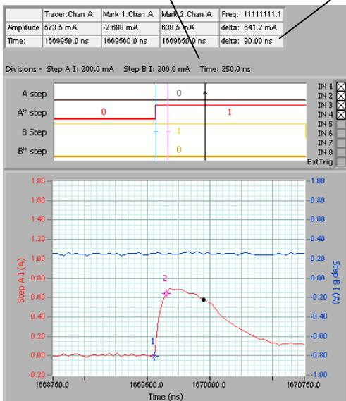
We can zoom all the way in to the limits of the current resolution (in this case 30ns) anywhere on the scope graph. Here we zoom on the single pulse shown in the tracking graph above.
