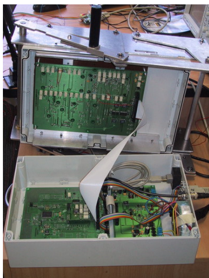
Here is a triple PCB test jig, using a Cleverscope and programmable Power Supply to carry out all test functions. In this example the Cleverscope is externally connected to allow re-use.
