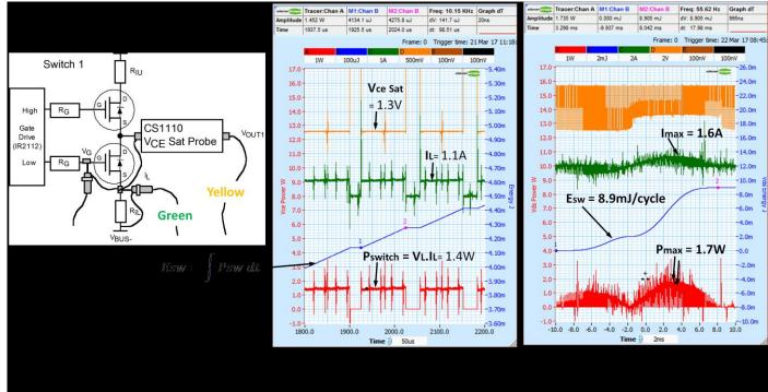
We use Maths to calculate the conduction current (green), the  $V_{CE}$  Sat probe to measure the switch saturation voltage (Yellow), the instantaneous power (red) and the energy per cycle (blue) to calculate the average conduction loss power (494 mW).
