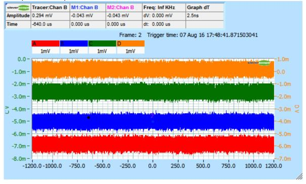
We use the signal information display to calculate the Standard Deviation (a good estimate of RMS, less the DC) and the peak to peak. We see less than 200uVrms noise, and less than 1.8mV p-p noise.
