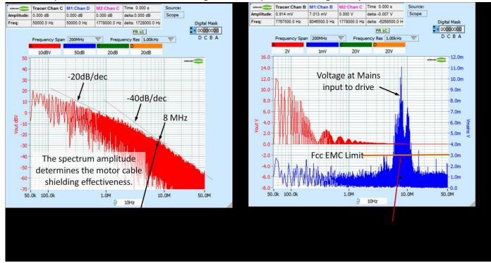
This test uses the Spectrum Analyser.
