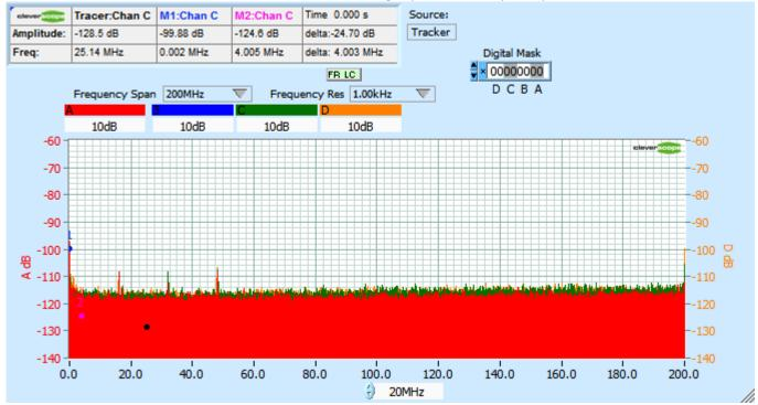
The three peaks are related to the front end processor 8 MHz clock. We will be working on reducing these.
