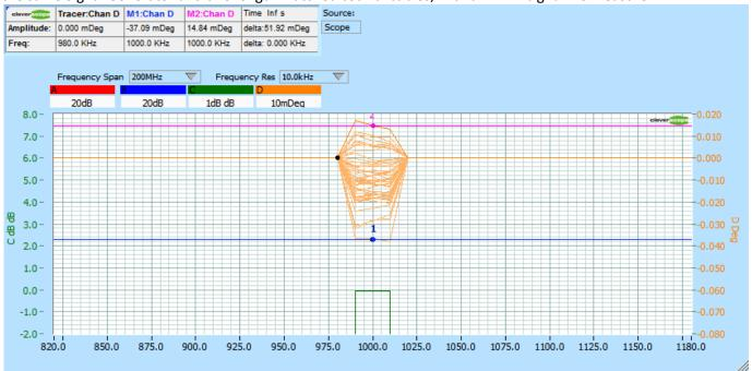
Persistence has been turned on to show the variability. We use Gain/Phase to make the measurement between Chans C and D. Gain was 0 dB. The phase varied from -0.037 deg to +0.015 deg, a variation of 0.052 deg at 1 MHz. This is the same as  $0.052/360 \times 1us = 144$  ps p-p variation. This is the same as 1 degree at 19.2 MHz.
