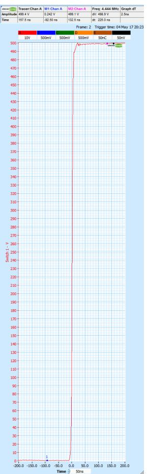
This trace shows the transition measured using a 100x probe. The display pixel resolution masks the actual channel resolution, shown here at 1V/div:
