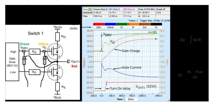
The high CMRR, and isolation allow making differential measurements across the gate drive resistor, even though it is swinging 325V in 37ns. Maths is used to calculate the gate current which is then integrated to calculate charge.
