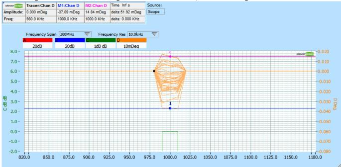
Persistence has been turned on to show the variability. We use Gain/Phase to make the measurement between Chans C and D. Gain was 0 dB. The phase varied from -0.037 deg to + 0.015 deg, a variation of 0.052 deg at 1 MHz. This is the same as 0.052/360 x 1us = 144 ps p-p variation. This is the same as 1 degree at 19.2 MHz.
