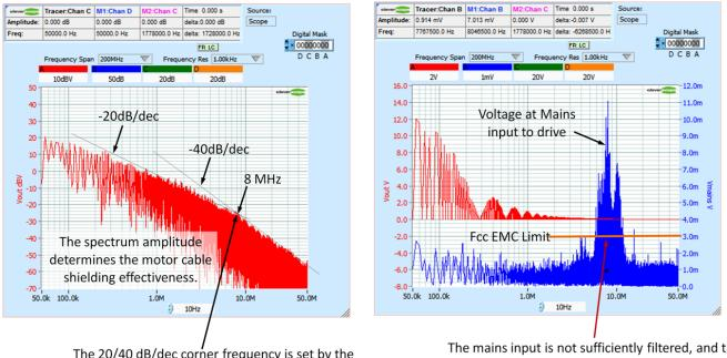
The 20/40 dB/dec corner frequency is set by the rise time (F =  $1/\pi$  37ns). A slower rise time reduces how good the shield needs to be.
