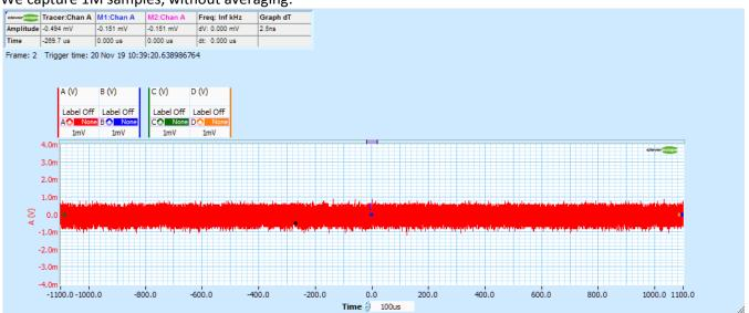
We use the signal information display to calculate the Standard Deviation (a good estimate of RMS, less the DC) and the peak to peak. We see about 200uVrms noise, and less than 1.8mV p-p noise.
