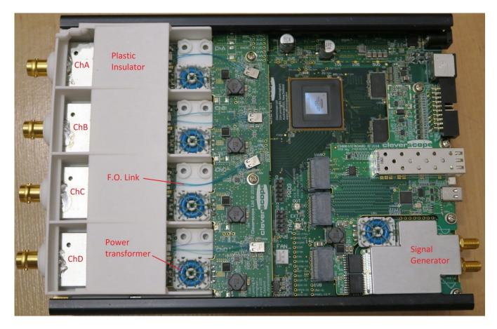
In this view (using a grey plastic insulating tray) we have omitted a transformer to show the separation.
