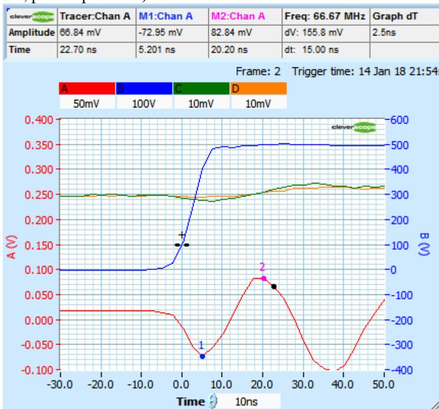
The oscillation period is about  $2 \times 15\text{ns} = 30\text{ns}$ , or  $f = 33 \text{ MHz}$ , so the inductance is a bit higher for this case (1.9uH), probably because the loop area is a bit bigger. The ring generates a differential end-to-end voltage along the length of the coax which is measured by the oscilloscope.
