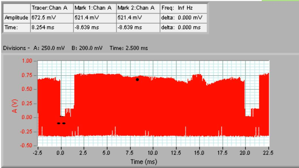
The trigger is the first pulse that meets the trigger specification.
