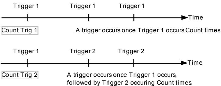
Each trigger definition provides a comprehensive mixed signal definition which provides triggering based on amplitude, duration and count.
