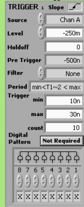
Here we have set up the triggers to catch all sync pulses whose rising edges take between 10 and 30ns to traverse
