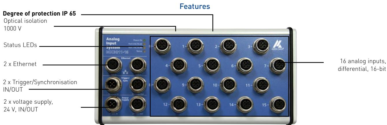
Ethernet, synchronisation and supply signals can be put through from one module to the next. In this way, you can acquire and process distributed I/O signals directly at production machines. These features allow the I/O modules to be used for simple, distributed applications and for complex applications, in which numerous devices have to interact with signals that are far away from each other.
