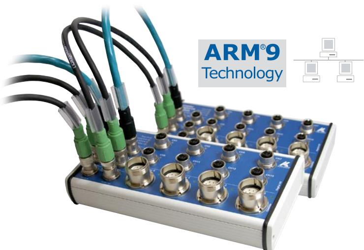
The intelligent Ethernet multifunction counter module MSX-E1701, MSX-E1711 and MSX-E1721 have 4 counter inputs for incremental or Sin/Cos encoders ( $1 \text{ V}_{\text{pp}}$  or  $11 \mu\text{A}_{\text{pp}}$ ) as well as 16 digital inputs and outputs, 24 V. The modules can be freely cascaded and synchronised in the  $\mu\text{s}$  range. You can thus acquire data from several modules at the same time. The ARM®9 processor allows to perform calculations.
