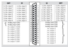
1: The analog inputs have a common ground line 2: Each analog output has its own ground line
