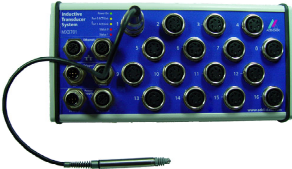
Fig. 5-8: Connecting transducers
