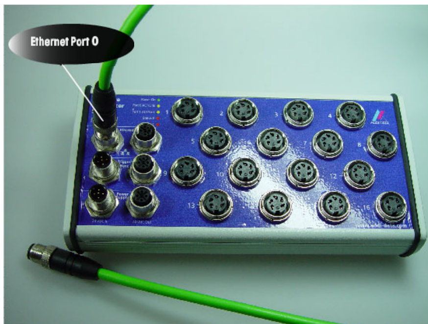
Fig. 5-9: Connecting Ethernet ports
