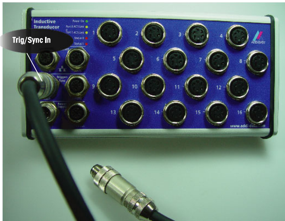
Fig. 5-10: Connecting trigger and synchro signals
