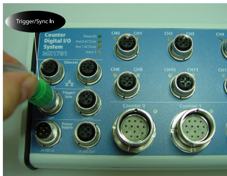
Fig. 5-9: Connecting trigger and synchro signals
