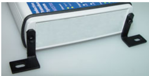
Fig. 5-3: Angles pointing to the outside
