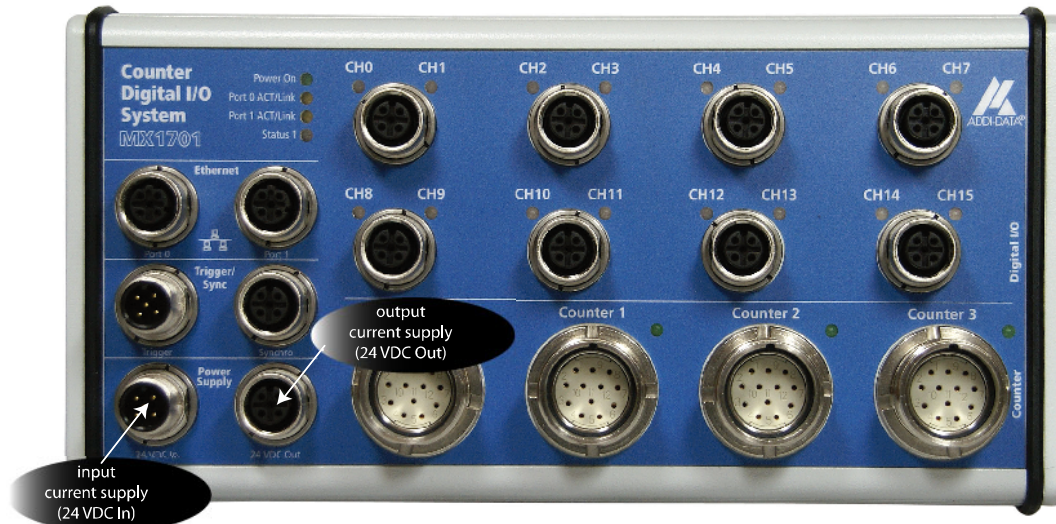
Fig. 5-10: Connecting the current supply
