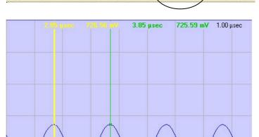
Two horizontal cursors are available, attached to Channel 1 only. The difference between both cursors is given at the right top corner in black color.
